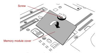
Figure 3-17 Seating the memory module cover
